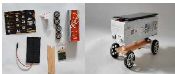
Figure 2. Volta Drive Connect Level 1 Design and Components
