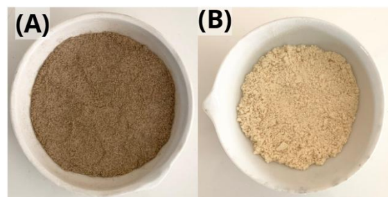
Figure 1. Physical appearance of (A) rice husk powder and (B) nanocellulose from rice husk
